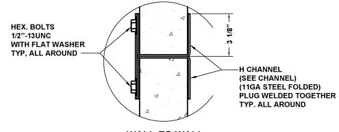
**WALL TO WALL SECTION PROFILE** \*IN THE CASE OF SECOND ROW OF WALL PANELS
